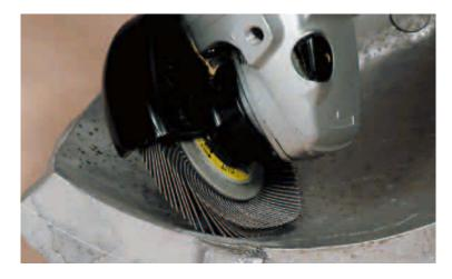
The use of a small substrate realizes curvature and flexibility of the abrasive cloth, which are suited to grinding/polishing tasks on curved or irregularly shaped surfaces.
